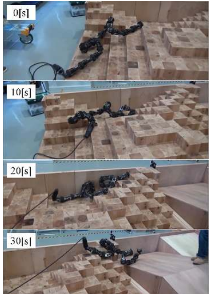
Fig. 17. Experimental result of the movement on a step field
