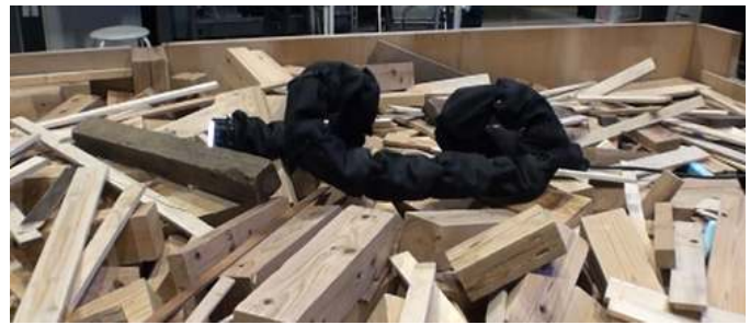
Fig. 16. Experimental result of the movement on a debris field
