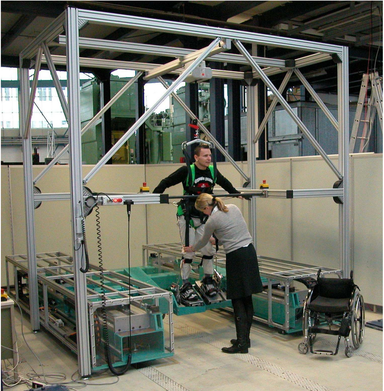
Figure 3 HapticWalker with SCI patient and physiotherapist. Photograph of the robotic walking simulator for gait rehabilitation HapticWalker.
