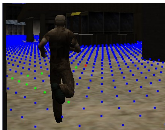
Fig. 11: The same level being navigated by a figure at run-time. The waypoints have been made visible for illustrative purposes. Most are blue, except for the green ones, which are part of the current path, and the red one, which is the goal.
