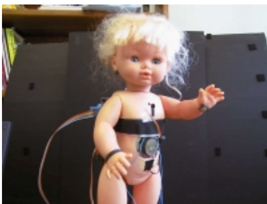
Figure 18.2. Robot, the humanoid robotic doll. The robot's dress is removed in order to show the robotic parts that control its movements.
