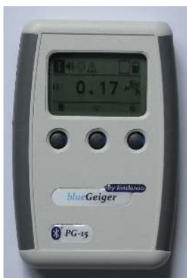
Figure 1. The BlueGeiger PG-15 dosimeter.
