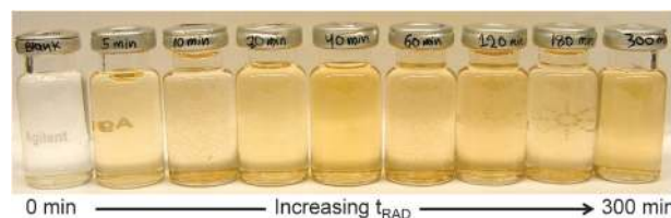
Fig. 2 Photographs of irradiated aerated solutions initially containing 0.3 \text{ mM CoSO}_4 at pH 10.6.
