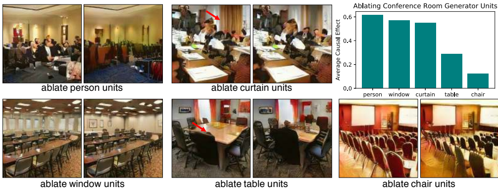
Figure 9: Measuring the effect of ablating units in a GAN trained on conference room images. Five different sets of units have been ablated related to a specific object class. In each case, 20 (out of 512) units are ablated from the same GAN model. The 20 units are specific to the object class and independent of the image. The average causal effect is reported as the portion of pixels that are removed in 1 000 randomly generated images. We observe that some object classes are easier to remove cleanly than others: a small ablation can erase most pixels for people, curtains, and windows, whereas a similar ablation for tables and chairs only reduces object sizes without deleting them.
