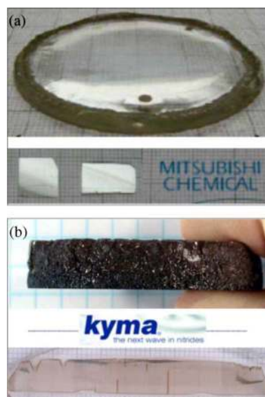
Fig. 2. The largest 2-in GaN boules reported currently by (a) Mitsubishi Chemical (adapted with permission from [49]) and (b) Kyma Technologies [13].
