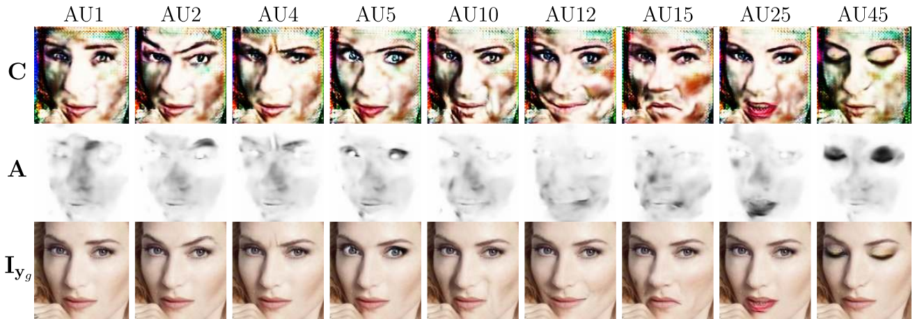
Fig. 5: Attention model. Details of the intermediate color mask C (first row) and the attention mask A (second row). The images in the bottom row are the synthesized expressions. Darker regions of the attention mask A show those areas of the image more relevant for each specific AU. Brighter areas are retained from the original image.
