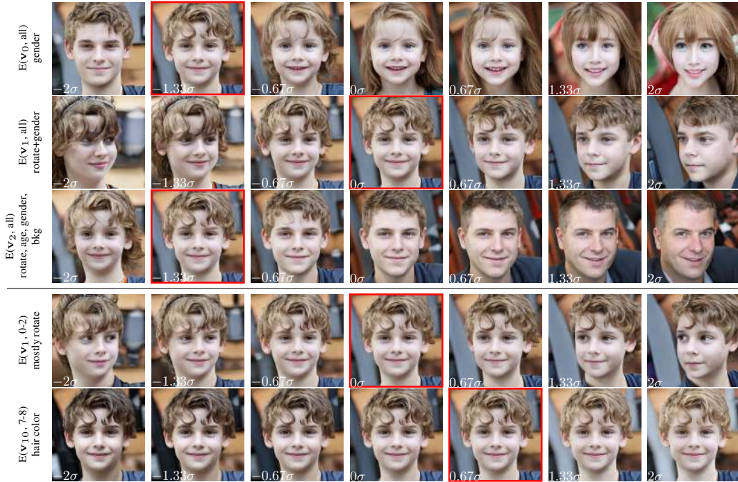
Figure 3: Rows 1-3 illustrate the three largest principal components in the intermediate \mathcal{W} latent space of StyleGAN2. They span the major variations expected of portrait photographs—such as gender and head rotation—with a few effects typically entangled together. The red square corresponds to location of the original image on each principal axis. Rows 4-5 demonstrate the effect of constraining the variation to a subset of the layers. For example, restricting the 2nd component to only layers 0-2, denoted E(\mathbf{v}_1, 0-2) , leaves a relatively pure head rotation that changes gender expression and identity less (compare to 2nd row). Similarly, selective application of the principal components allows control of features such as hair color, aspects of hairstyle, and lighting. See SM §1 for a larger sampling.
