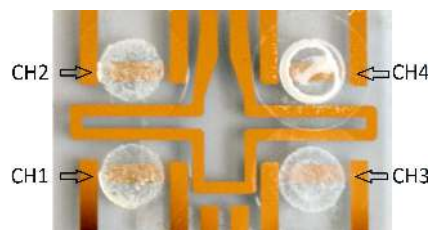
Fig. 5. Ready sensor made from nanoparticles on comb electrodes. CH1 – TiO 2 350; CH2 – TiO 2 450; CH3 – ZnO A; CH4 – ZnO B
