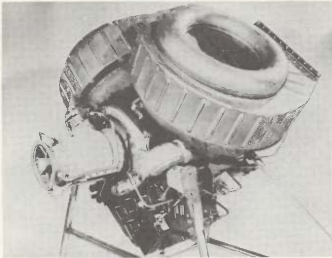
Fig. 20 Recuperative gas turbine for helicopter propulsion
