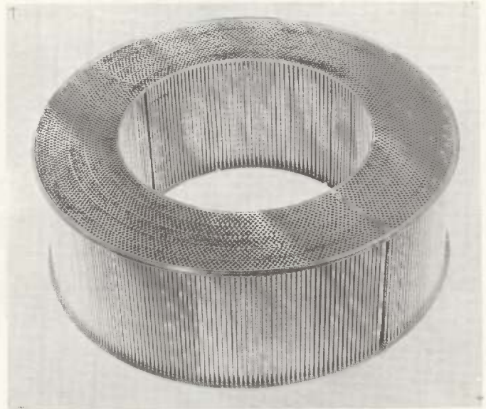
Fig. 21 Compact, lightweight tubular recuperator matrix
