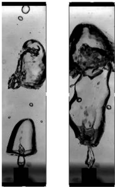
Gas flow rate Q_g : 36 cm 3 /s Gas flow rate Q_g : 80 cm 3 /s
