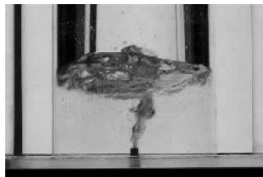
Fig. 1. Swirl motion of a bottom blown bath. (Liquid: water, gas: air, vessel diameter D : 200 mm, bath depth H_L : 100 mm, gas flow rate Q_g : 100 cm 3 /s, inner nozzle diameter d_{ni} : 2.0 mm)
