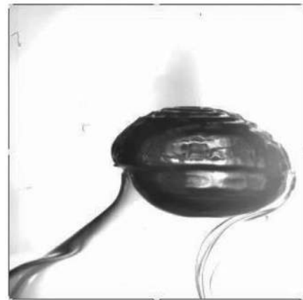
Fig. 20. Propagation of interfacial tension wave on a bubble rising in silicone oil layer. (front view, d_B=8.31 mm, v_m=v_s=1.00 \times 10^{-6} m 2 /s, \sigma_{ms}=0.0527 N/m, t_0 : initiation time of interfacial tension wave, Uemura et al. 44 )
