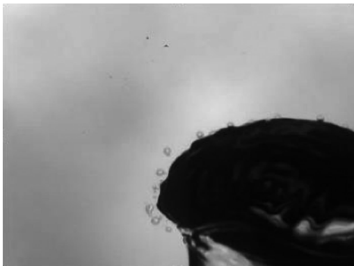
Fig. 22. Magnified view of a bubble and fine water droplets caused by interfacial tension wave, Uemura et al. 44 .
