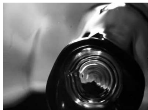
Fig. 21. Interfacial tension wave on a bubble rising in silicone oil layer. (top view, d_B=8.31 mm, v_m=v_s=1.00 \times 10^{-6} m 2 /s, \sigma_{ms}=0.0527 N/m, t_0 : initiation time of interfacial tension wave, Uemura et al. 44 )
