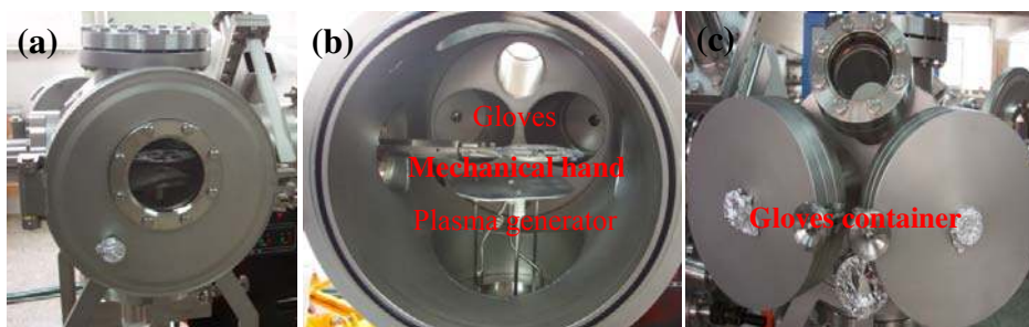
Figure 3-2.(a) Front, (b) Inside and (c) Back view of pretreatment chamber.
