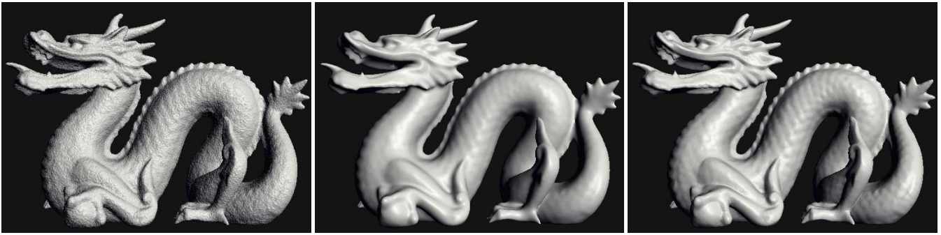
Figure 10: Non-local means for geometry smoothing. Left: the dragon model corrupted by Gaussian noise with \sigma = 1/2 mean edge length Middle: smooth base layer produced by Laplacian smoothing of the noisy mesh; Right: non-local means result. This mesh contains 300K vertices and it took under a minute to perform the denoising.
