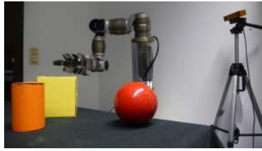
Fig. 7. Experimental setup: Schunk 7DoF arm, Schunk 7DoF hand, Bumblebee stereo camera, coloured objects with various shapes.
