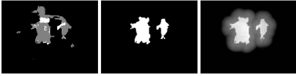
Figure 3. Left is the initial labeling of foreground regions (white), background regions (black), and unlabeled regions (gray). Middle is the final binary labeling of foreground and background regions. Right is the final content map M .
