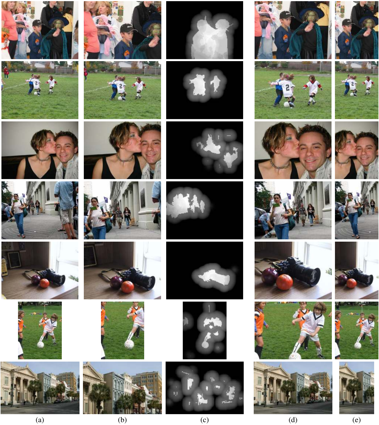
Figure 6. Results for a set of representative images. (a) Original image; (b) fully automatic crop [Suh et al. 2003]; (c) gaze-based content map; (d,e) gaze-based crops to horizontal and vertical aspect ratios.
