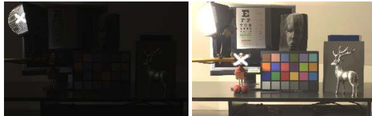
Fig. 2. Images viewed by an observer adapted to different areas of the scene indicated by the white crosses. In the left image the adaptation luminance is close to 1790 \text{ cd/m}^2 , in the right to 5 \text{ cd/m}^2 .
