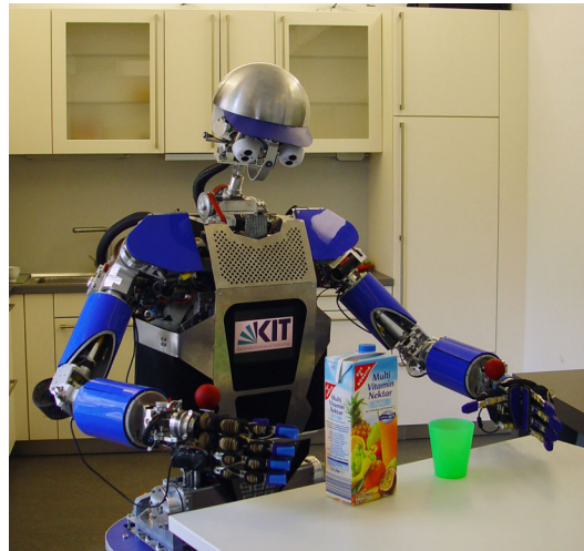
Fig. 1. ARMAR-IIIa [1] performing bimanual visual servoing in order to pour juice into a cup. During this task, both target objects as well as the hands of the robot need to be observed by the visual system. Due to the large workspace, the selection of appropriate gaze directions is required in order to cover all task relevant objects and thus allow successful execution of the task.
