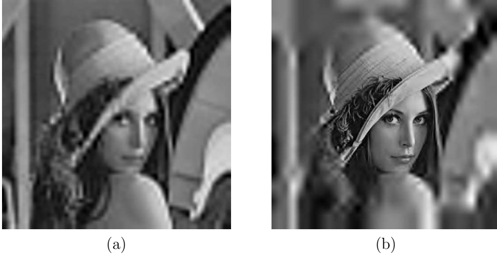
Fig. 1. Reconstructed ‘Lena’ image at 0.125 bits per pixel (bpp) for (a) JPEG 2000 and (b) JPEG 2000 based region of interest (ROI) prioritisation method.
