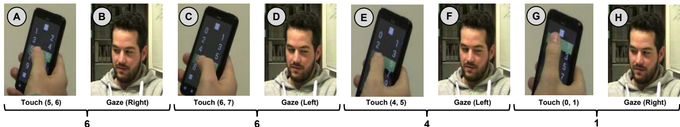
Figure 1: We propose using gaze and touch for authentication on smartphones when accessing sensitive data. GazeTouchPIN is robust against shoulder surfing since it requires attackers to observe the user’s eyes and the touchscreen simultaneously. In the example the user enters “6641”. Users first select a row of two digits via touch, then gaze left or right to determine the digit to select. To complicate shoulder surfing, one of two digits layouts is randomly chosen at every entry (e.g., compare A to C).
