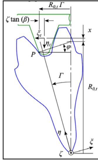
Figure 2 Helical gear conjugated to its basic rack.
