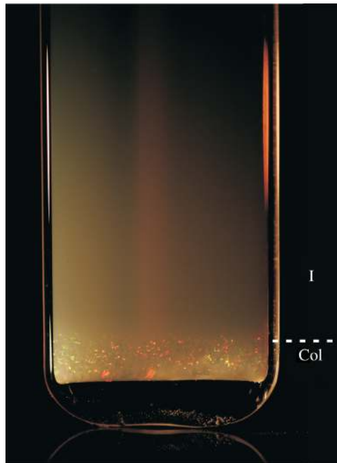
Figure 4. Photograph of a 100 \text{ g dm}^{-3} sample at 10^{-4} \text{ M} , illuminated by white light. The top part is isotropic (I), while the bottom part is columnar (Col) as is revealed by the presence of Bragg reflections. The photograph is taken 2.5 years after preparation.
