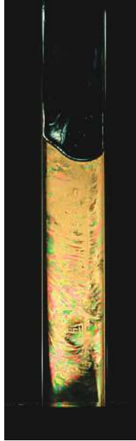
Figure 3. Photograph of 200 \text{ g dm}^{-3} gibbsite at 10^{-4} \text{ M} between crossed polarizers, 2.5 years after preparation.
