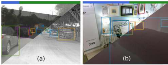
Fig. 1. Output samples of the proposed multi-modal object detector. The blue/green bar at the top illustrates the contribution/reliability of each sensor modality in obtaining the final output. Images from two modalities are merged diagonally only for illustration purposes. (a) Shows the results on the FLIR-Thermal dataset with RGB and thermal sensor modalities, (b) Shows the output on the SUNRGB-D dataset with RGB and our proposed “r-blended” hybrid depth modality.
