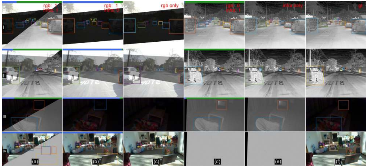
Fig. 5. Qualitative analysis of our multi-modal object detector, g_{sa} in this case. Columns (a), (b) and (d) are the outputs of g_{sa} in various asymmetric sensor failure conditions imitated artificially, which are mentioned on the upper-right corner of each image in row I. The top blue/green bars represent the contribution of each sensor modality in obtaining the final results (RGB: blue and Thermal/Infra: green). (c) and (e) are the outputs from single modal baselines. (f) is the ground-truth. Rows I and II are from FLIR-Thermal dataset while III and IV are from L515-Indoor dataset. Row IV represents a true sensor failure case when IR camera gets saturated due to sun-light even in indoors.
