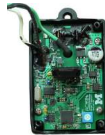
(a) Voltage Monitor
