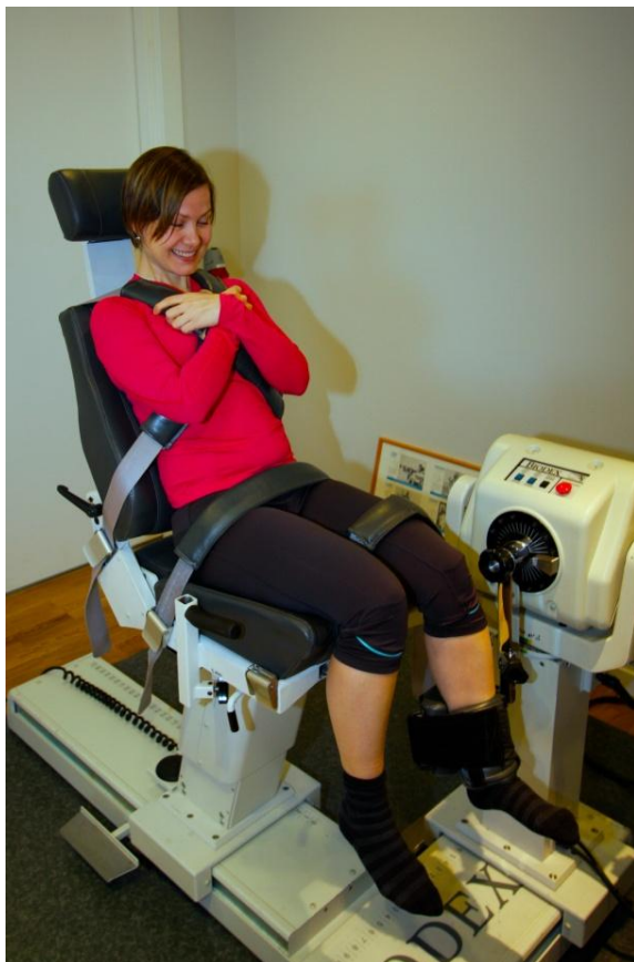
Fig. 6 Isokinetic muscle testing of the thigh muscles with a Biodex dynamometer. (Photo: Fredrik Eklund)
