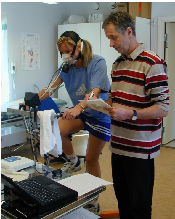
Fig. 7 Ergospirometry during an incremental cycle ergometer test
