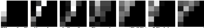
Fig. 6: Radius-based Surface Descriptors (RSD): 2D histograms of normal angle difference and distance from a reference point to its neighbors (examples are shown from left to right for histograms computed for points on a plane, sphere, corner, edge and three cylinders, where the last two are computed for different points of the corrected teapot scan presented in Figure 4) – from these histograms the physical surface radii can be read as the slopes of the different lines going through the lower left corners.
