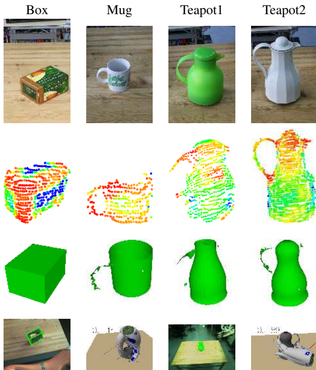
Fig. 8: Automatic modeling applied to various objects. 1st row: objects on kitchen table, 2nd row: radius estimation results on the reconstructed point cloud (for the interpretation of the colors please see Figure 4), 3th row: generated geometric models, 4th row: applications to grasping and matching in 2D images
