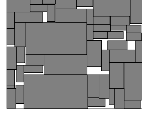
Fig. 5. Placement of MCNC benchmark: ami49. Achieve total area of 37,935,800, and total wire length of 2,761,122 in 1.52 hours on Sun SPARC 20 workstation. The result is the average of 15 runs. Notice that we didn't compare our result with [6] because the current implementation of our approach uses cost function. The final result has to be affected by the coefficient in the cost function.
