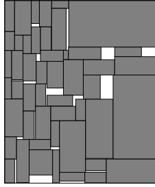
Fig. 4. Floorplanning of MCNC benchmark: ami49 given each block is soft. Achieve total area of 37,334,668 (%3.9 improvement) and total wire length of 2,893,677 in 2.28 hours on Sun SPARC 20 workstation. The result is the average of 10 runs.
