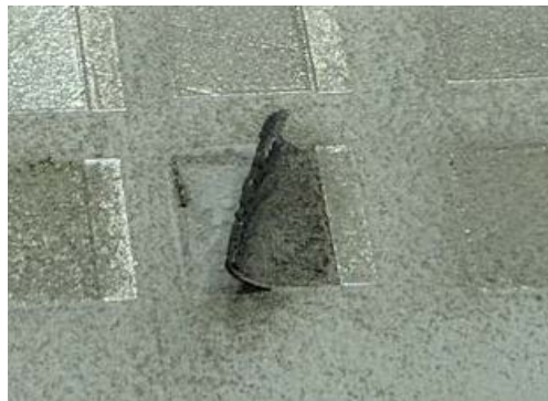
Figure 5: The consequence of large residual stress
