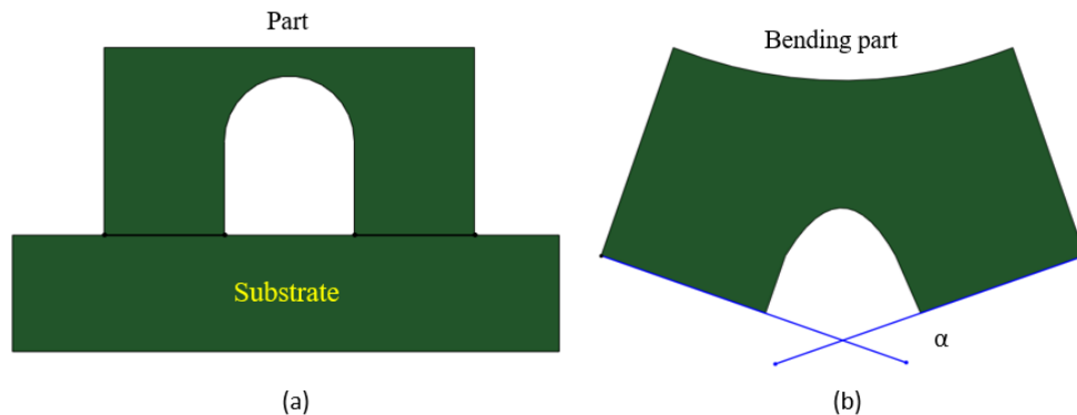
Figure 6: (a) Before, (b) after removal from the base plate. The geometry of the test parts
