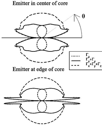
FIG. 5. Spontaneous emission as a function of the off-axis angle for an emitter in the center of the core and an emitter at the edge of the core of a step-index fiber with  $n_1=1.45$ ,  $n_2=1.43$ ,  $a=2 \mu\text{m}$ , and for  $\lambda_0=1560 \text{ nm}$ .
