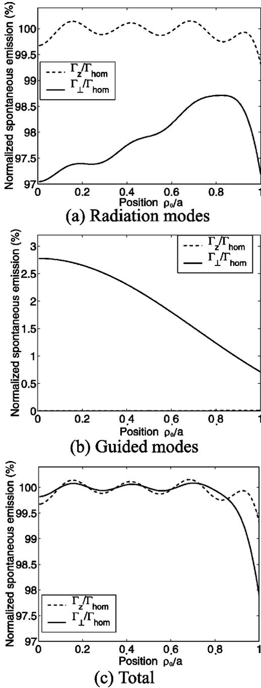
FIG. 2. Spontaneous emission as a function of position for an emitter in the core of a step-index fiber with core refractive index  $n_1=1.45$ , cladding refractive index  $n_2=1.43$ , and core radius  $a = 2 \mu\text{m}$ . The emission wavelength is  $\lambda_0=1560 \text{ nm}$ .
