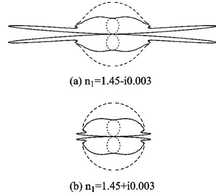
FIG. 6. Spontaneous emission as a function of the off-axis angle for an emitter at the edge of the core of a step-index fiber with  $a=2 \mu\text{m}$ ,  $n_2=1.43$  and (a)  $n_1=1.45-i0.003$ , (b)  $n_1=1.45+i0.003$ , and for  $\lambda_0=1560 \text{ nm}$ .
