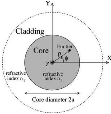
FIG. 1. Illustration of the circular step-index optical fiber with core refractive index  $n_1$ , cladding refractive index  $n_2$ , and core diameter  $2a$ . A Cartesian coordinate system  $(x, y, z)$  is introduced with the origin placed in the center of the fiber core, and with the fiber oriented along the  $z$  axis. The position of a point source is given by  $(\rho, \phi, z)$ .
