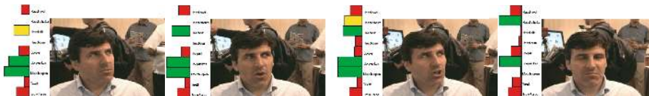
Fig. 2. Real time display recognition (frames sampled every 0.7s). The bars represent the output probabilities of the HMM classifiers (top to bottom): head nod, shake, tilt, turn, lip corner pull, lip pucker, mouth open, teeth and eye-brow raise.
