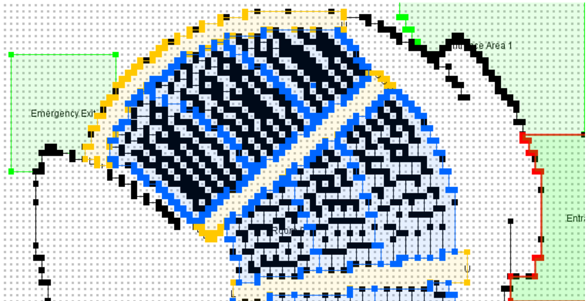
Figure 3.2: A model of a lecture hall within the editor of ZET. The building geometry is visualized by black lines. Assignment areas are denoted in blue, green represents evacuation areas and stair areas are depicted in yellow.
