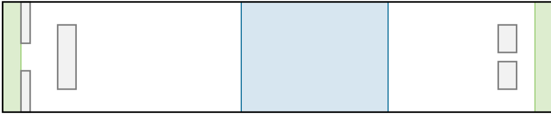
Figure 3.8: Two exits with different kinds of obstacles in front of them. The pillars on the right side allow for a narrow path such that evacuees will not take the detour around the obstacles.
