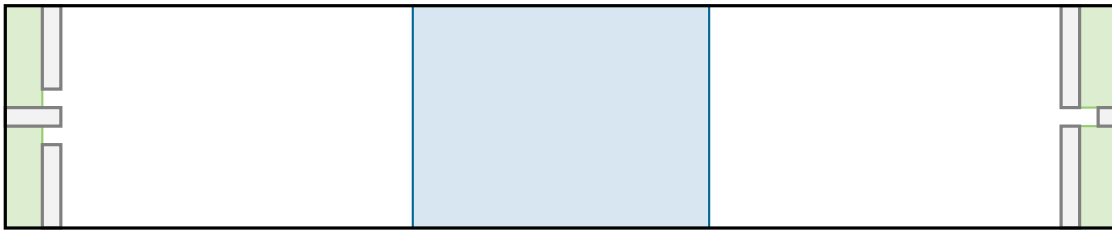
Figure 3.9: Four exits on two opposite sides. The exits on the left side each have a unique entry while the two exits on the right side share a single bottleneck.
