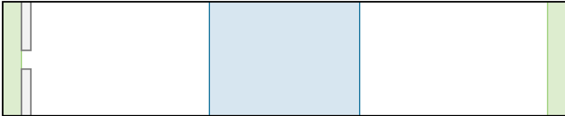
Figure 3.6: Test scenario with two exits (in green) of different capacity. The evacuees reside exactly in between the exits in the blue area.
