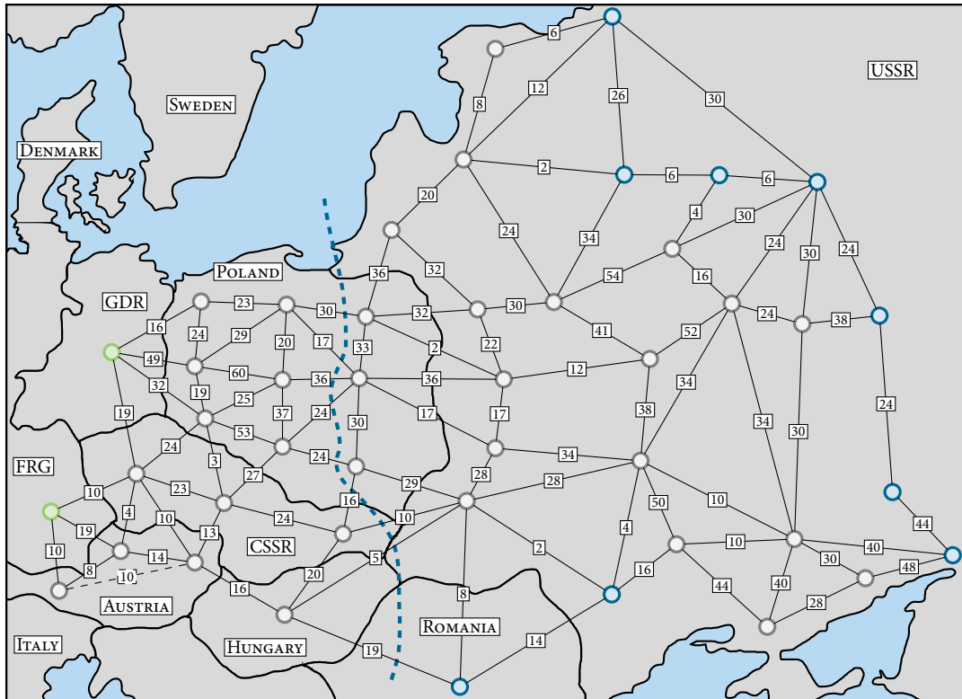
Figure 1.1: The Soviet rail network used as motivational example for the start of network flow research by Ford and Fulkerson. The dashed line represents the minimum cut.
