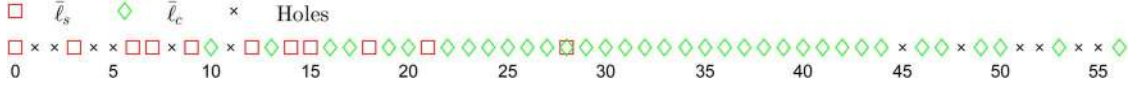
Fig. 6. An example of CADiS configuration coarrays, where p = 2 , \check{M} = 3 , N = 7 and L = \check{M} + N .
