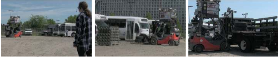
(a) Photographs of the forklift executing the command, “Put the tire pallet on the truck.”
