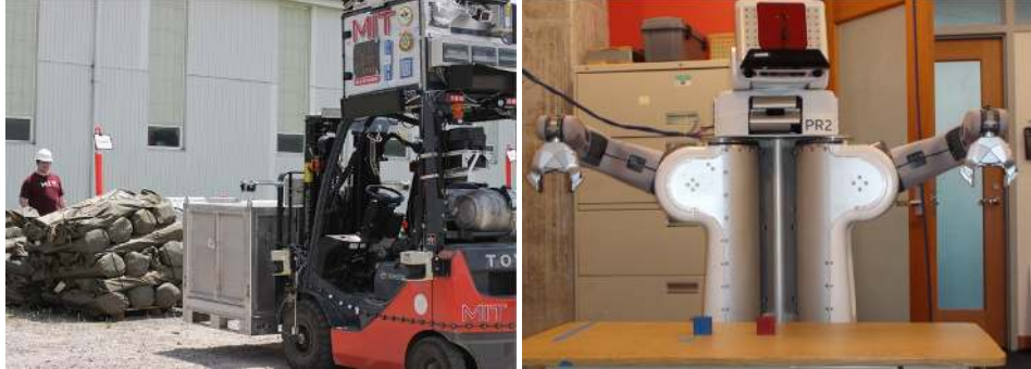
(a) Robotic forklift, operating in an outdoor (b) PR2, a mobile humanoid operating in indoor, household environments.
