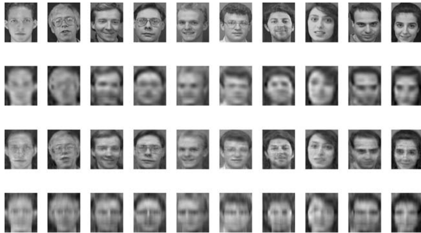
Figure 8. First row: raw images from ORL dataset. Second row: images compressed by GLRAM. Third row: images compressed by SVD. Fourth row: images compressed by 2DPCA. Note that the compression ratio of SVD (3.85) is much smaller than that of GLRAM (98.0).
