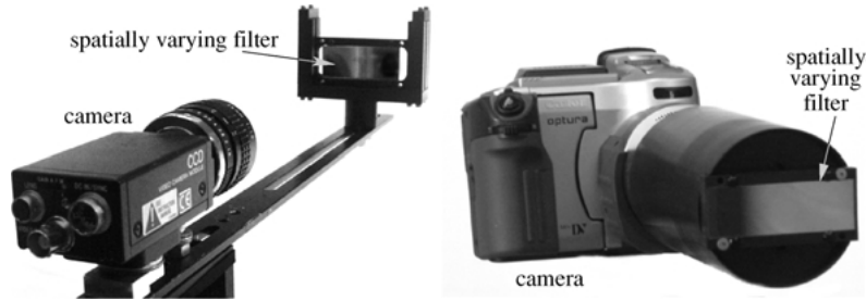
Figure 3. Two generalized mosaicing systems. (Left) A system composed of a Sony black/white video camera and an extended arm which holds the filter. (Right) A system that includes a Canon Optura digital video camera and a cylindrical attachment that holds the filter. In both cases, the camera moves with the attached filter as a rigid system.
