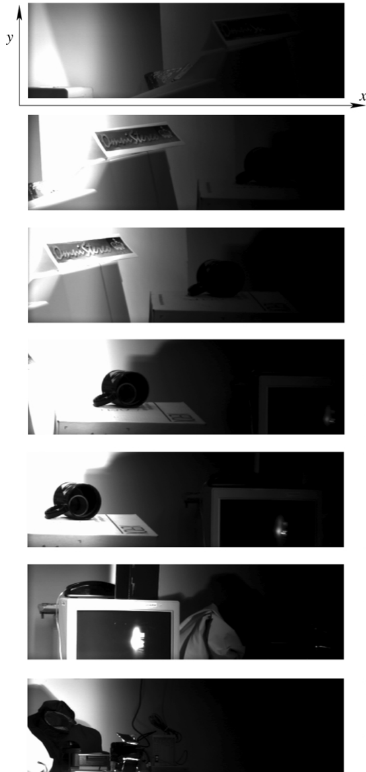
Figure 11. Frames 4, 9, 11, 15, 17, 23, and 31 from a sequence taken with a linear variable density filter. Scene features become brighter as they move leftwards in the frame. Bright scene points gradually reach saturation. Dim scene points, which are not visible in the right hand side of the frames, become visible when they appear on the left.
