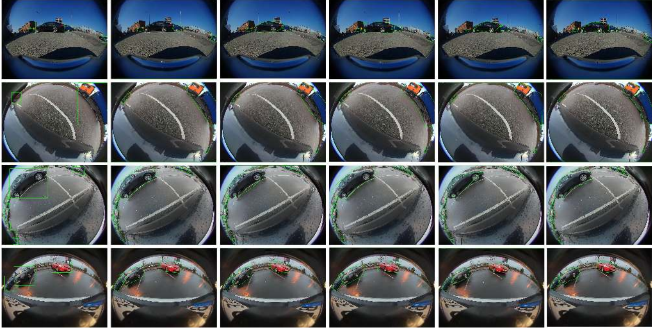
Figure 7: Qualitative results of the proposed model outputting different representations. Rows represent front, left, right, and rear camera images, respectively. From left to right: Standard box, Oriented box, Ellipse, Curved box, 4-point polygon, 24-point polygon.
