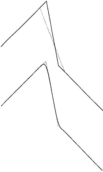
Figure 13. Smoothing the gaps by linear interpolation, then extending the blocks somewhat into the gaps, then smoothing with a sigmoid function.
