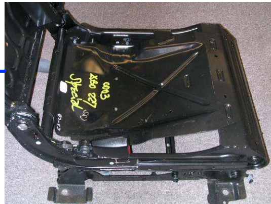
Rigid Seat Pan Multi-piece stamped and welded steel pan (No foam or cover shown)
