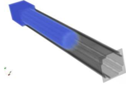
FIG. 7. Capillary intrusion of water into a single cylindrical pore initially filled with hexane, i.e., \rho_I/\rho_O = 1.5094 and \mu_I/\mu_O = 3.2277 . The water-solid contact angle is 40^\circ and t^* \approx 48.3 .
