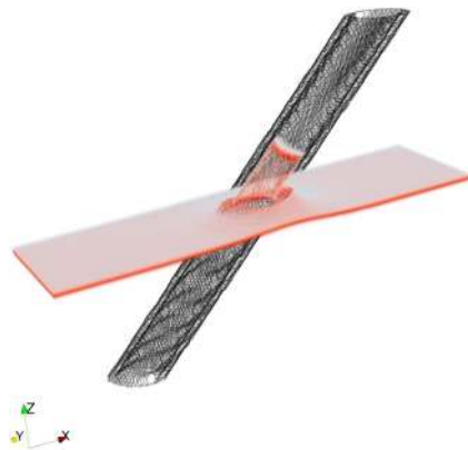
FIG. 5. Graphical representation of the rotated tube geometry with the bottom fluid highlight. As predicted by Jurin's law, the capillary rise is clearly visible. Note that the lattice resolution s = 2 , the viscosity ratio \nu_B/\nu_T = 20 , the Laplace number La = 10 , the contact angle \theta_c = 45^\circ , and the geometry rotations (\theta_x, \theta_y, \theta_z) = (30^\circ, 30^\circ, 30^\circ) .
