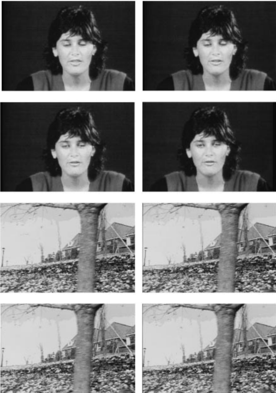
Fig. 9. Quantized image sequence for nonadaptive VQ for 4-D vectors ( 2 \times 2 tiles) and a local codebook of 256 codewords (MSE = 234.9, rate = 1.487 b/pixel).
