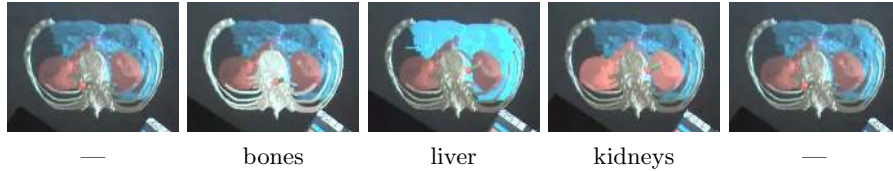
Fig. 12. Several snapshots from a video which was taken through a session where the user moved a 3D pointing device across a 3D dataset of a human chest in a virtual environment. Visual object high-lighting reflects the current 3D position of the 3D pointing device which is very useful to efficiently position the device in 3D space during object selection.
