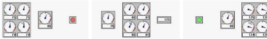
Fig. 15. F+C process visualization: depending on where the user points, the virtual instruments are drawn at a smaller or larger level of detail (from left to right: the pointer is moved from left to right).
