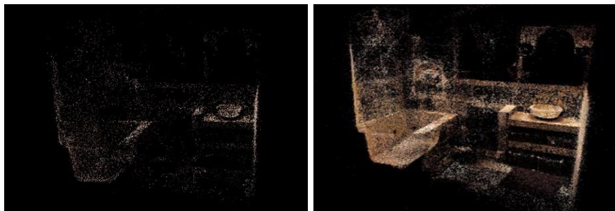
Figure 13: A sample of the generated PCD for indoor settings: bathroom- Sparse PCD
