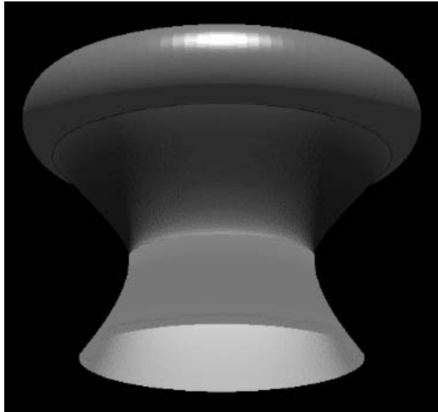
Fig. 7. The blending surface between a circular torus and a hyperboloid of one sheet
