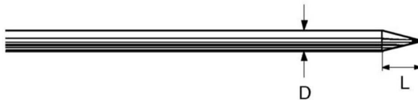
Figure 21 The tip of the electrode is ground to a length L=1.5-2 times the diameter ( D ) (Weman , 2012)
