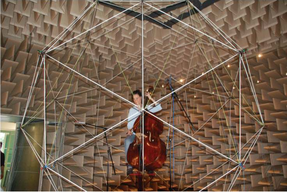
FIG. 6. (Color online) Spherical microphone array surrounding the musicians.
