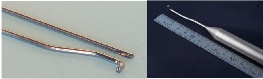
Fig. 6 4-hole cobra probe manufactured and calibrated by Turbulent Flow Instruments ( http://www.turbulentflow.com.au/ )
