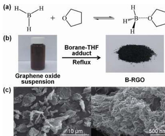
Figure 1. (a) A borane–THF adduct, (b) a reaction scheme of the reduction of graphene oxide with the borane–THF adduct, (c) SEM images of B-rG-O powder at different magnifications.
