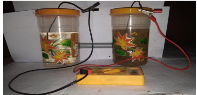
Figure 1: Microbial Fuel Cell for the treatment of waste water
