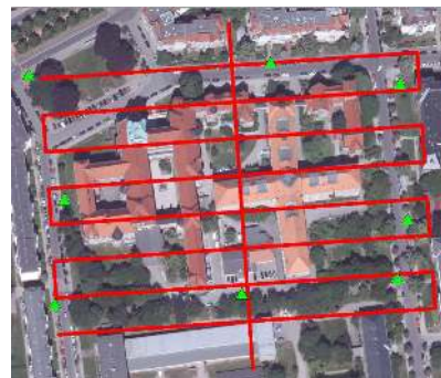
Figure 2. Planned flight path (red line) and positions of control points (green triangles) orthophoto data source: ATKIS®-DOP © Staatsbetrieb Geobasisinformation und Vermessung Sachsen 2013
