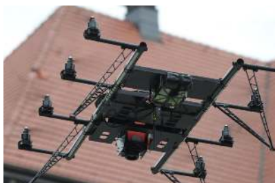
Figure 1. Horus octocopter equipped with thermal infrared camera InfraTec mobileIR E9 and RGB camera GoPro HD Hero
