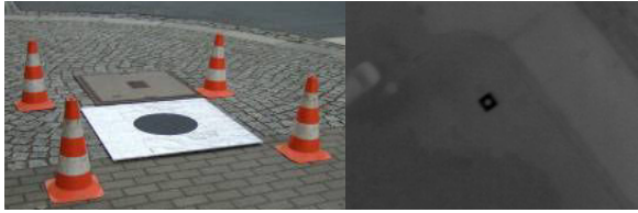
Figure 3. Control points (left: RGB image; right: thermal image from 150 m height)
